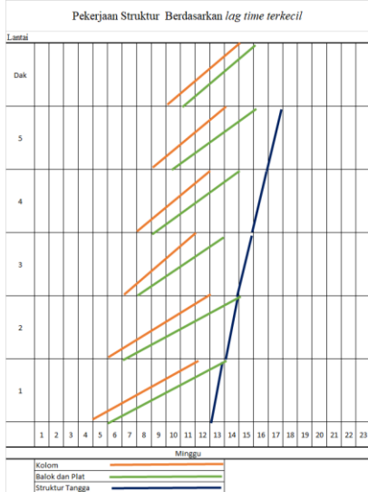
Figure 3 Line of Balance Diagram for Structural Work Based on Minimum Lag Time
