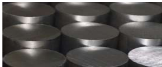
Figure-6. AISI 4140 steel material diameter dimensions D=30
