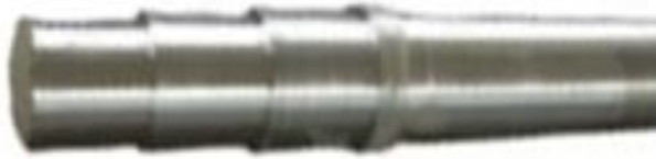
Figure-4.Axle rail shafts material of AISI 4337 Steel Standard Conditions of workpieces with a length / diameter ratio greater than 10 are not recommended (ISO 3685).
