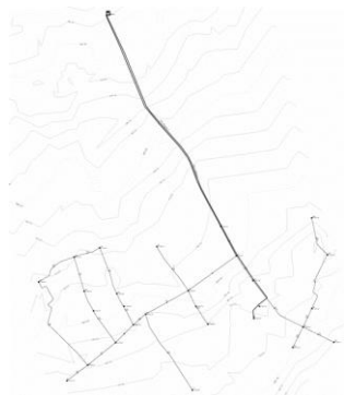
Figure 8. Visualization of the Umbulan Spring Distribution Pipeline Network Table 11 Umbulan Spring Flow Rate Output Results (Peak Hours)
