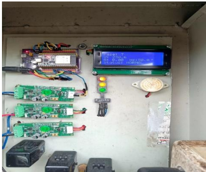
Figure 3 Phase T normal condition
