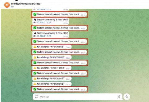
Figure 4 Normal condition notification
