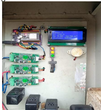
Figure 2 Phase S normal condition
